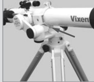
b) Interference with the optical tube in vertical direction.
