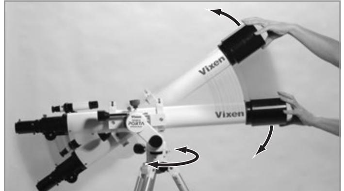
Note: The tension of the friction stop motion can be adjusted in the altitude and azimuth directions as the need arises.
