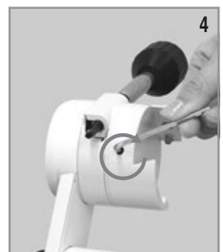
**5** Replace the lock screw and attach the optical tube to the dovetail mounting block to finish.
