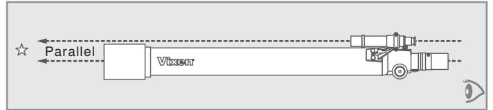
**Be sure to align the finder scope with the telescope's field of view before you start observing. It is highly recommended to do this in daytime.**
