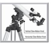
(Note) The slow-motion knobs turn within the limited range. If you want to turn them further, loosen the vertical / horizontal motion clamp
