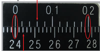
Example 1 Vernier 0.02mm Increments
