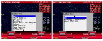
Choose Rec. Start in the PEC screen and press Select to start recording while you confirm the guide star is in the center of the cross hairs. Continue tracking the guide star until the recoding completes. Since your manual operations are recorded exactly, you need to implement the corrections as precisely as possible. The process takes 8 minutes in full circle.
