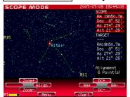
Press Menu to display the System Menu. Move the cursor to PEC with the ↑ keys and press Select to enter the PEC screen.
