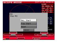
\*If the PEC recording is done over one cycle, Play Start will be shown underneath the indication of Rec. Start. If the PEC recording is less than one cycle, Play Start won't be indicated.
