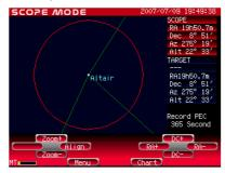
During the PEC recording, the guide star may begin slipping out in the direction of the tracking (in the direction of RA). Use the RA+, RA- keys to keep the guider star at the center of the cross hairs.
