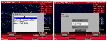
\*If the PEC recording is done over one cycle, Play Stop will be shown on the screen. If the PEC recording is less than one cycle, Rec. Stop will be indicated.
