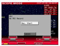
On starting the recording the screen is automatically zoomed to the maximum. You can zoom down for the wide screen with the Zoom – key, but be sure to set the zoom level at the maximum when you make the correction. Corrections may be useless in other zoom levels.
