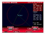
\*The motor control on the mount is set at the slowest rate during the play back of the PEC recording and you cannot slew the telescope with the RA+, RA-, DC+, DC- keys quickly. Cancel the play back if you need to slew the telescope at higher speed. Automatic Go-To slewing is possible during the play pack.
